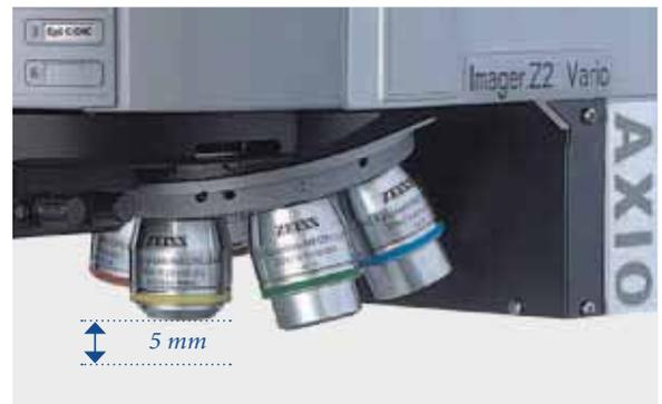
The sample is brought into focus simply by moving the nosepiece up and down.
